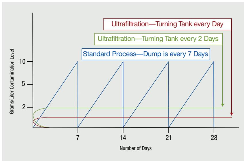
**Figure 2: Comparison of contamination levels in a typical aqueous cleaning system and a cleaning system with UF.**
