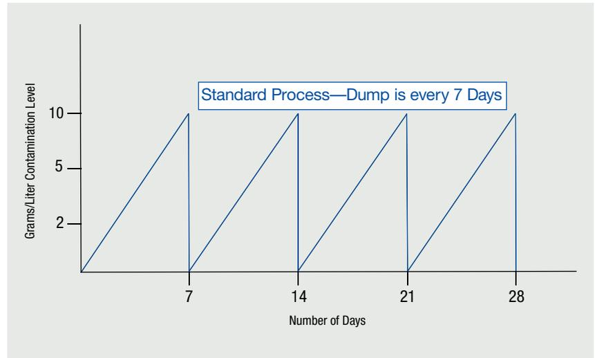
Figure 1: Typical aqueous cleaning process without ultrafiltration.
