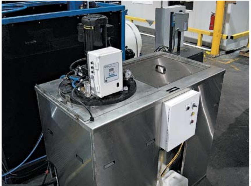
Deerfield Manufacturing installed a 360 gal./day UF system that effectively turns over its wash tank every fourth day.
