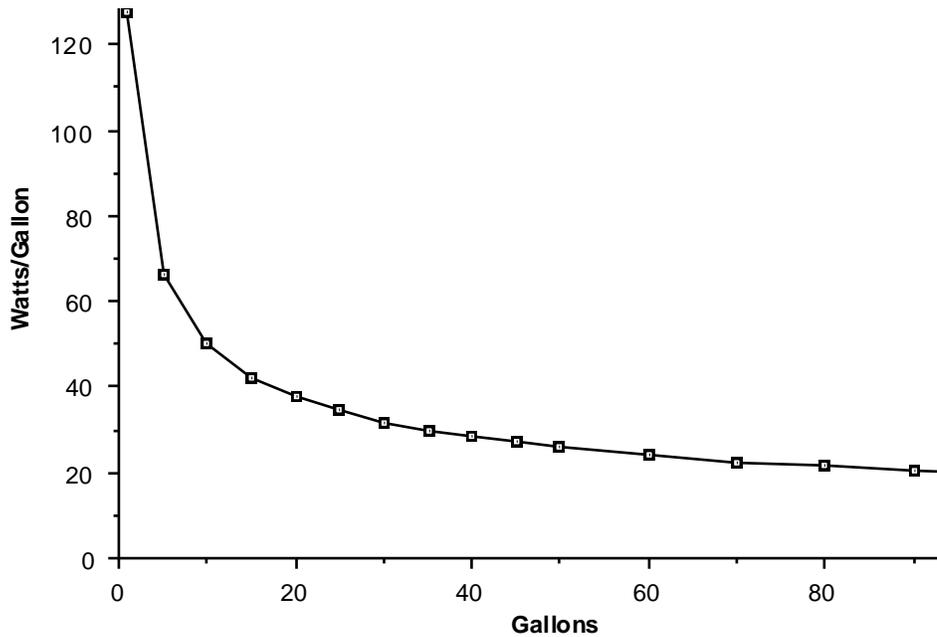
This curve was generated by taking a number of known successful installations and fitting a curve to the data. As tank capacity is extended further, the number of watts per gallon required continues to decrease at a diminishing rate.
